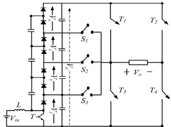
Fig.9. Proposed 9-level power electronic converter structure.
