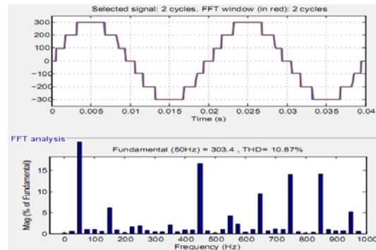
Fig. 7. Output voltage and harmonic spectrum of 7-Level power electronic converter (THD=10.87%).
