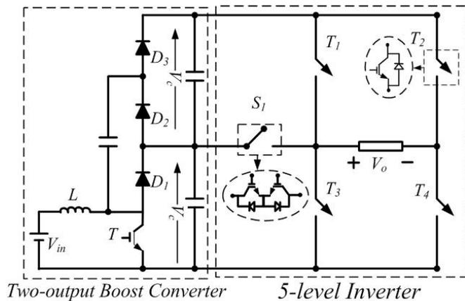
Fig. 2. Basic unit for proposed power electronic converter topology.
