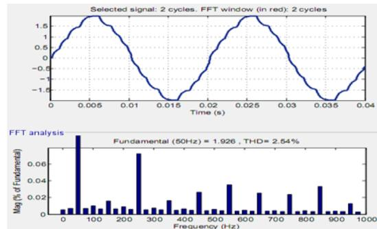
Fig. 12. Output current and harmonic spectrum of 9-level power electronic converter (THD=2.54%).
