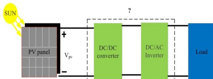
Fig. 1. The structure of photovoltaic systems.
