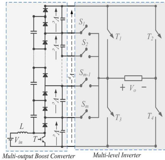
Fig. 4. Proposed power electronic converter (PEC).
