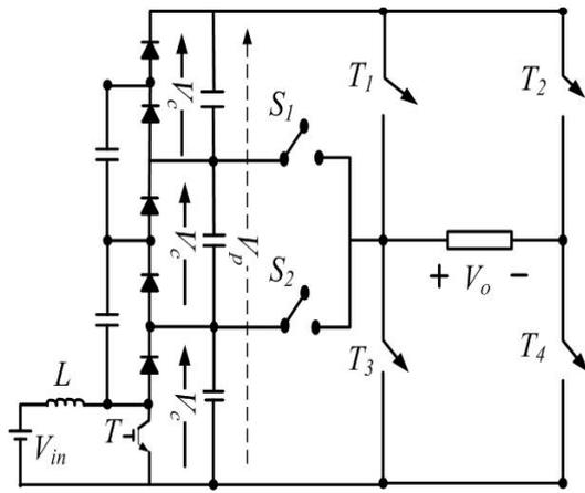
Fig. 5. Proposed 7-level power electronic converter structure.
