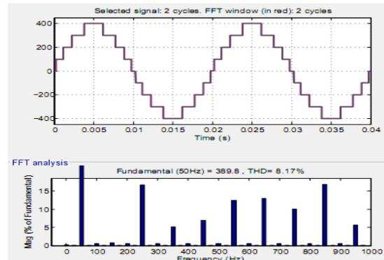
Fig. 11. Output voltage and harmonic spectrum of 9-Level power electronic converter (THD=8.17%).
