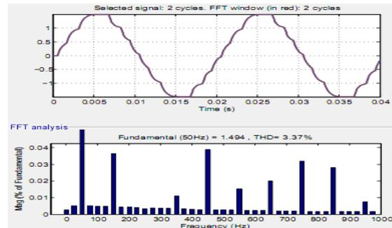
Fig. 8. Output current and harmonic spectrum of 7-level power electronic converter (THD=3.37%).
