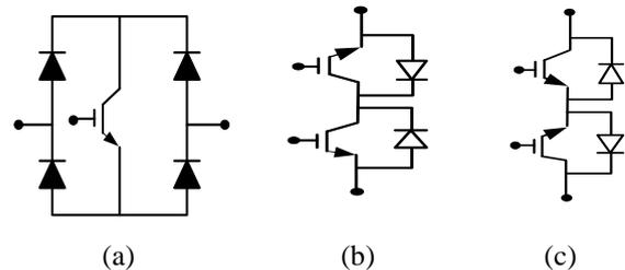
Fig. 3. Different structures for bidirectional switches.
